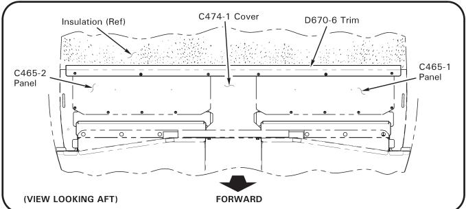
FIGURE 36-2 AFT CABIN ACCESS PANELS
