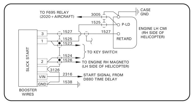
Figure 3A R44 II SS1002 SlickSTART® Schematic
