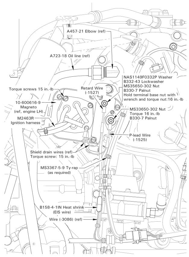
Figure 7 R44 II CMI magneto installation, engine LH shown (View looking aft; R44 similar)
