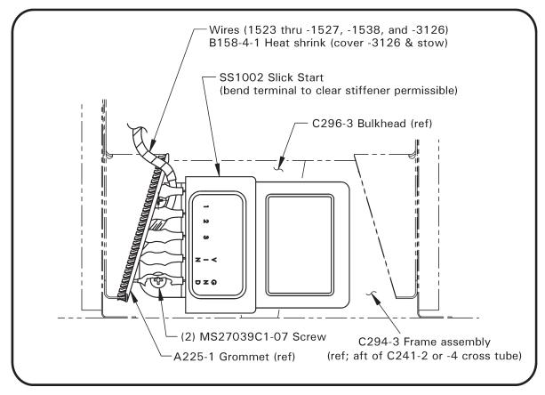
Figure 2A R44 II SS1002 SlickSTART® installation (aft seat tunnel; view looking forward)
