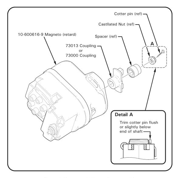
Figure 6 Magneto 73013 coupling assembly
