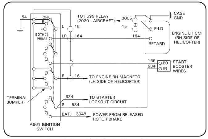
Figure 3B R44 and Cadet Starting Vibrator Schematic
