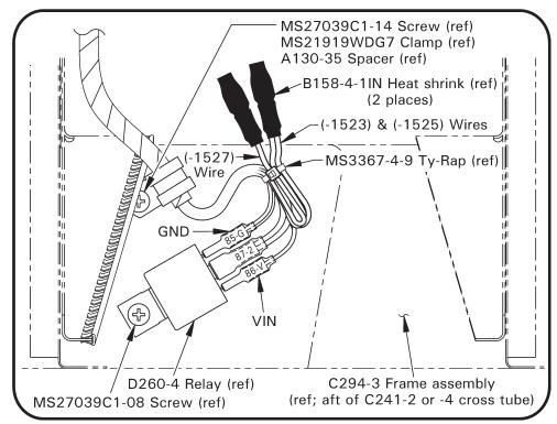
Figure 1 D260-4 Relay installation location (aft seat tunnel; view looking forward)
