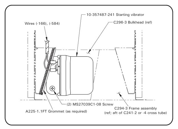
Figure 2B R44 & Cadet Starting Vibrator Installation (aft seat tunnel; view looking forward)
