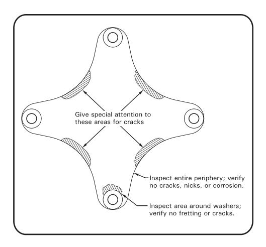
FIGURE 5-4A FLEX PLATE INSPECTION
