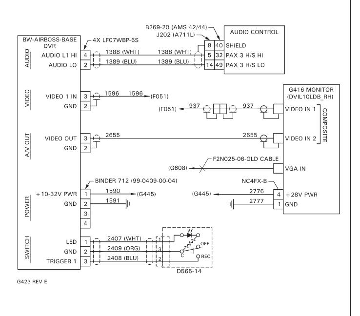
FIGURE 90-13 G415-1 AND G416-4 AND MONITOR INSTALLATION WIRING SCHEMATIC
