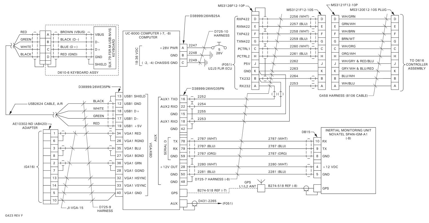
FIGURE 90-18 G608 GPS MAPPING AND MDT INSTALLATION WIRING SCHEMATIC
