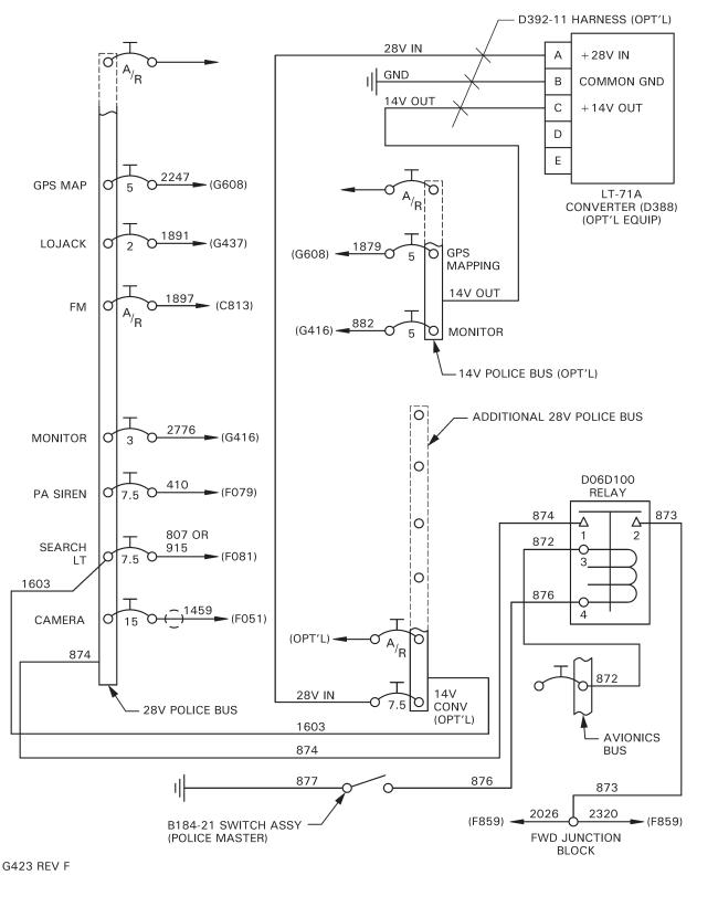
FIGURE 90-16 G445 AND G467 AUX ELECTRICAL AND CB WIRING INSTALLATION WIRING SCHEMATIC
