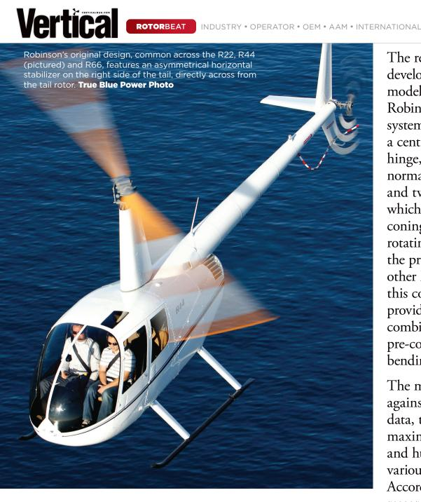
The researchers developed a simulation model specifically for Robinson's tri-hinge rotor system, which includes a central teetering hinge, responsible for normal blade flapping, and two coning hinges, which accommodate the coning motion of the rotating blades due to the production of lift. In other helicopter models, this coning action is provided for through a combination of a fixed pre-cone angle and blade bending.
