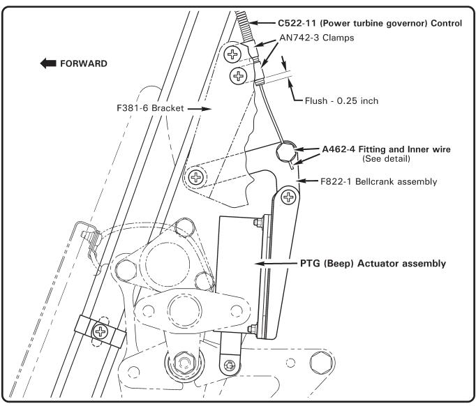
FIGURE 76-3 PTG (BEEP) ACTUATOR ASSEMBLY
