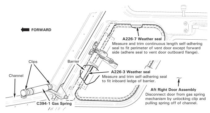
FIGURE 52-2 GAS SPRINGS AND DOOR VENTS
