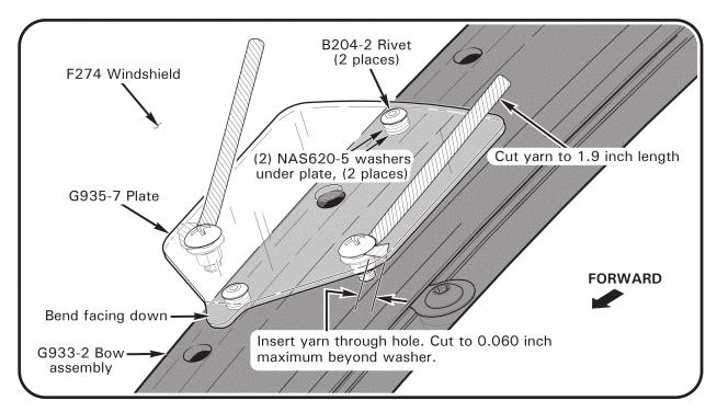
FIGURE 52-6 G935-7 PLATE INSTALLATION
