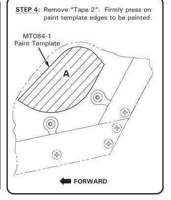
FIGURE 52-5 PAINT TEMPLATE LAYOUT PROCESS
