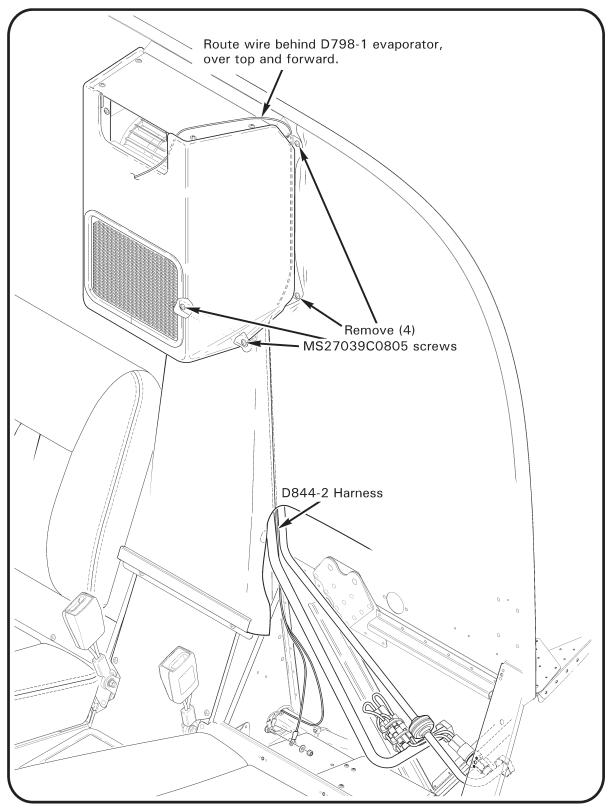
FIGURE 3 location for D844-2 harness wiring (view looking aft, inboard)
