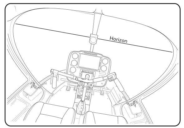
FIGURE 6 Camera view angle (angle shown requires adjustment)
