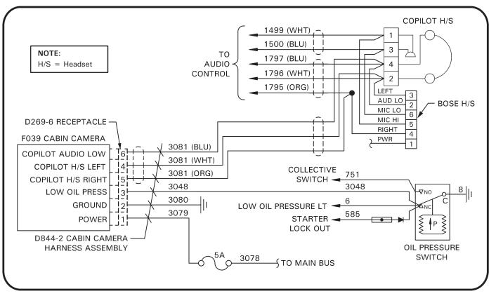
**FIGURE 1 Wiring schematic** (typical; see MM § 14.00 for additional wiring diagrams)
