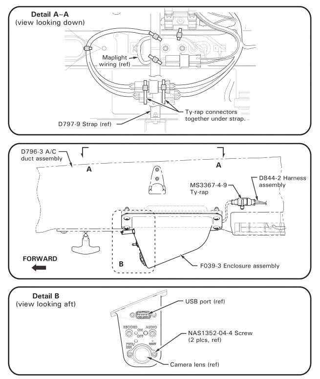
FIGURE 2 Connecting camera to D844-2 harness
