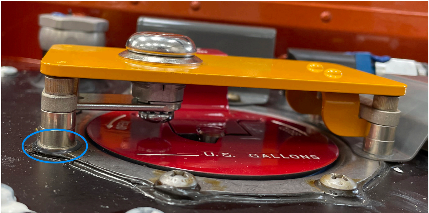
FIGURE 3 B270-1 sealant applied to cover top side (F250-10 cover shown; F250-1 similar)
