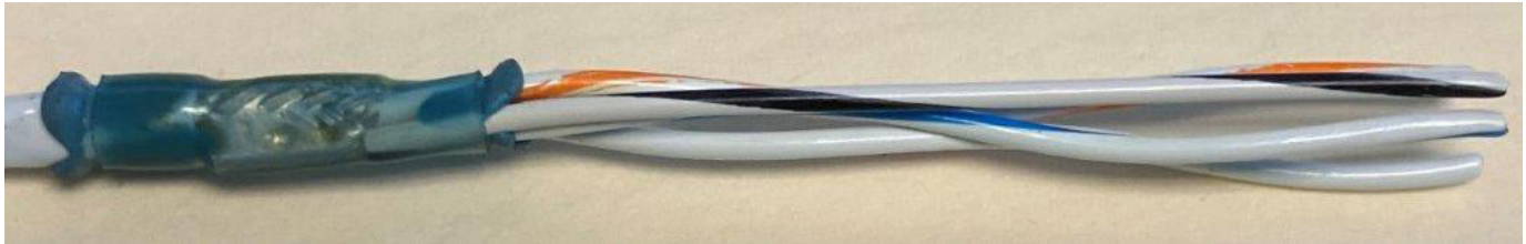
FIGURE 8 Proper installation of terminator
