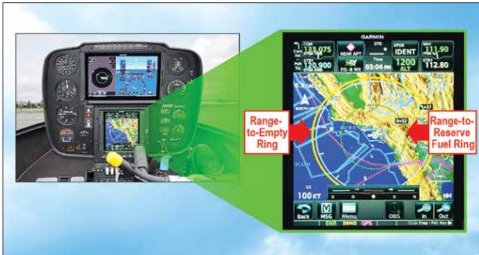
Fuel flow data displays on the Garmin GTN 750Xi.
