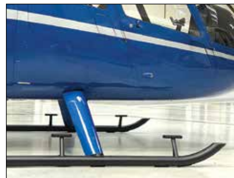
Steps installed on the R66.
