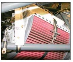
Inlet Barrier Filter installed in R66
