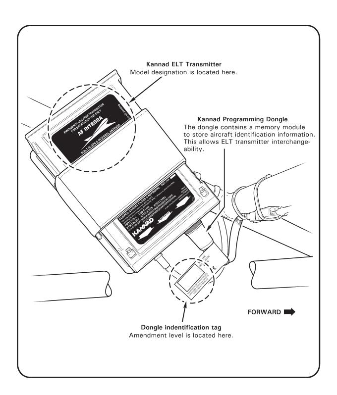
FIGURE 1 KANNAD ELT AND DONGLE INSTALLATION (R44 Shown)
