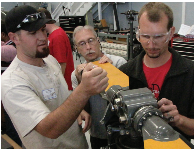
Students Norman, Lill, and Brown learn a main rotor mast maintenance task.
