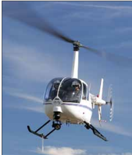
Baton Rouge's new police helicopter features a FLIR camera, Lojack, searchlight and P/A speaker.
