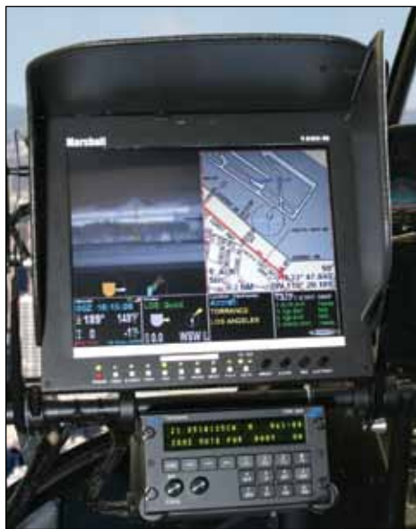
AeroComputers' split-screen shows FLIR image of a building (left) and building's map location (right).
