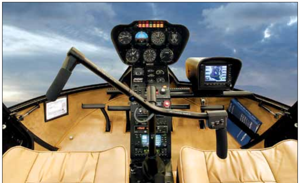
The R66 Turbine Cockpit (shown with 7-hole instrument panel and optional Pilot's Avionics Console).
