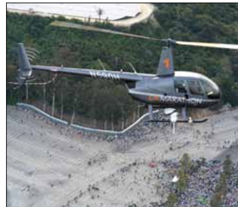
Raven IIs relayed microwave signals from camera trucks to a transmitter truck.
