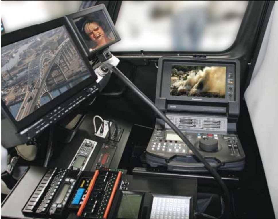
The R44 Newscopter's passenger/ENG workstation shown with optional Panasonic P2 Mobile HD recorder.
