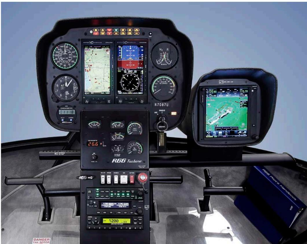
8-Instrument Console with Pilot Avionics Console
