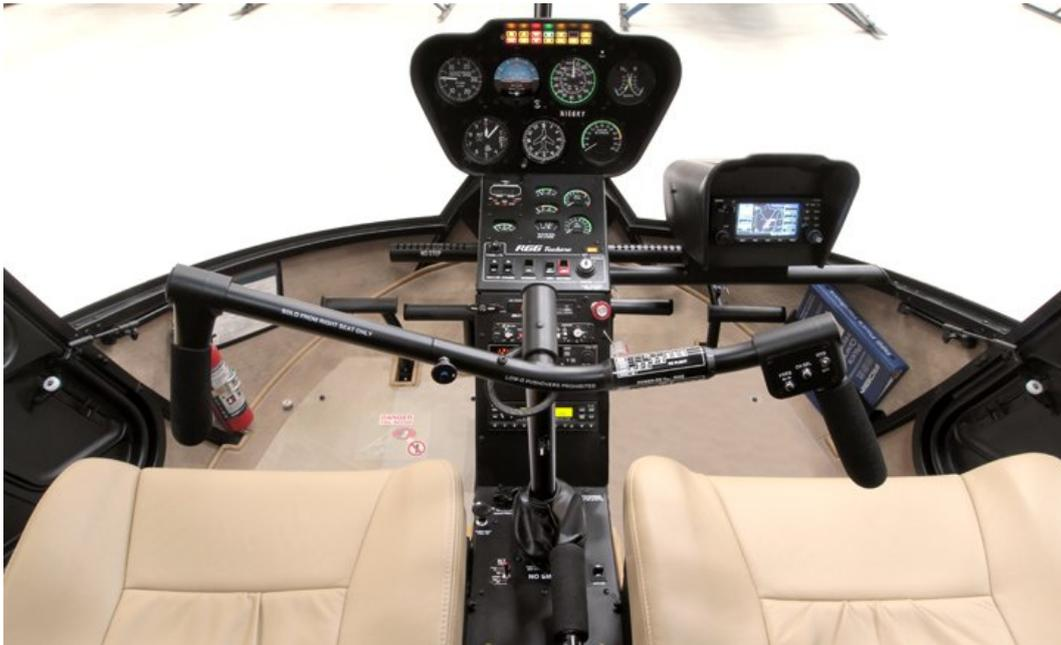
Original 7-Instrument Console with Pilot Avionics Console
