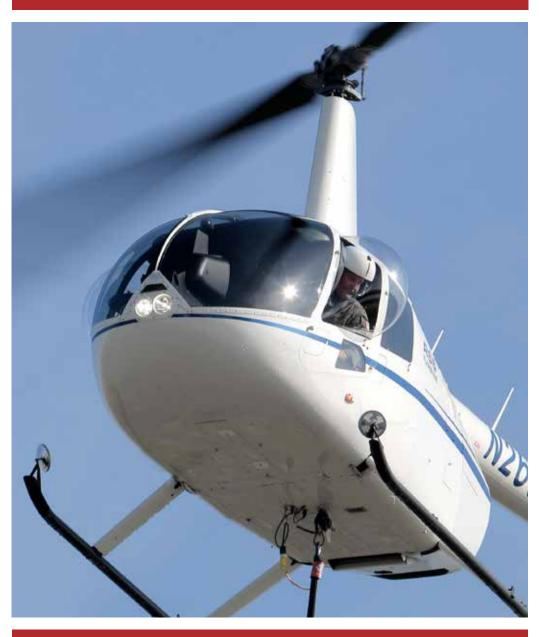
The R66 Turbine helicopter cargo hook installation provides maximum utility for external load operations in a light, single-engine helicopter. Using a proven Onboard Systems hook, the R66 installation is rated for external loads up to 1200 lb with a maximum combined helicopter plus load weight of 2900 lb (up from the normal 2700 lb).
