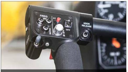
The cargo hook kit includes an upgraded left side cyclic grip with external load control and hook release switches as well as hydraulic switch and radio controls.
