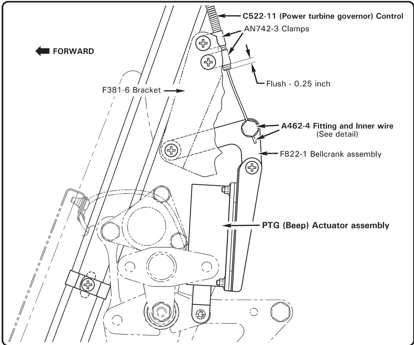
**FIGURE 76-3 PTG (BEEP) ACTUATOR ASSEMBLY**
