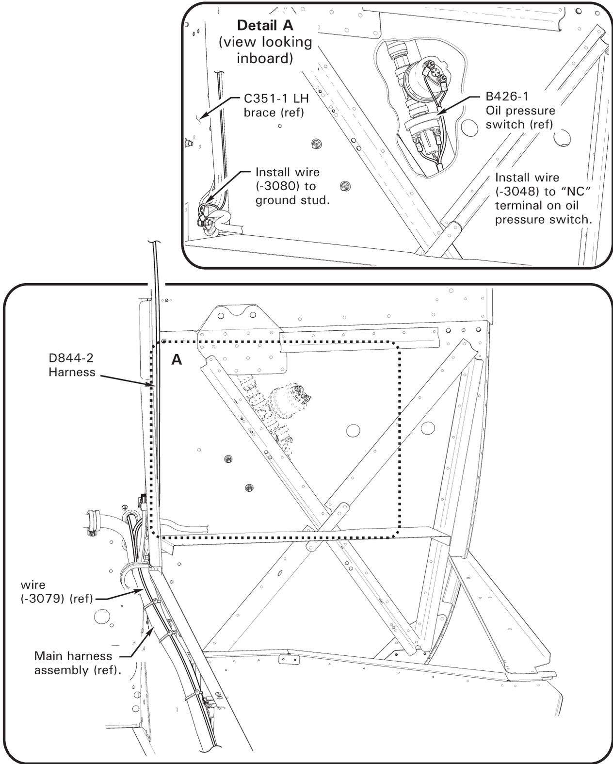
**FIGURE 4** Terminating locations for D844-2 harness wiring
