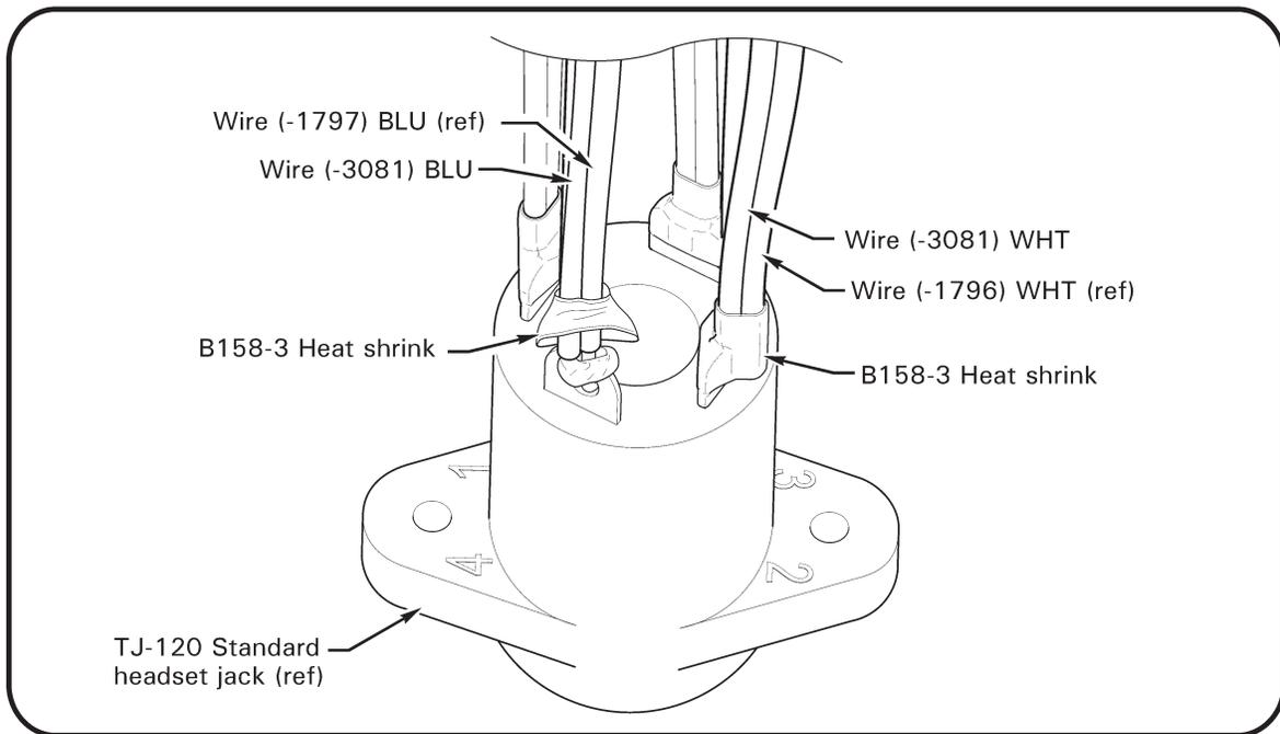
**FIGURE 1A Solder splice at TJ-120 jack**
