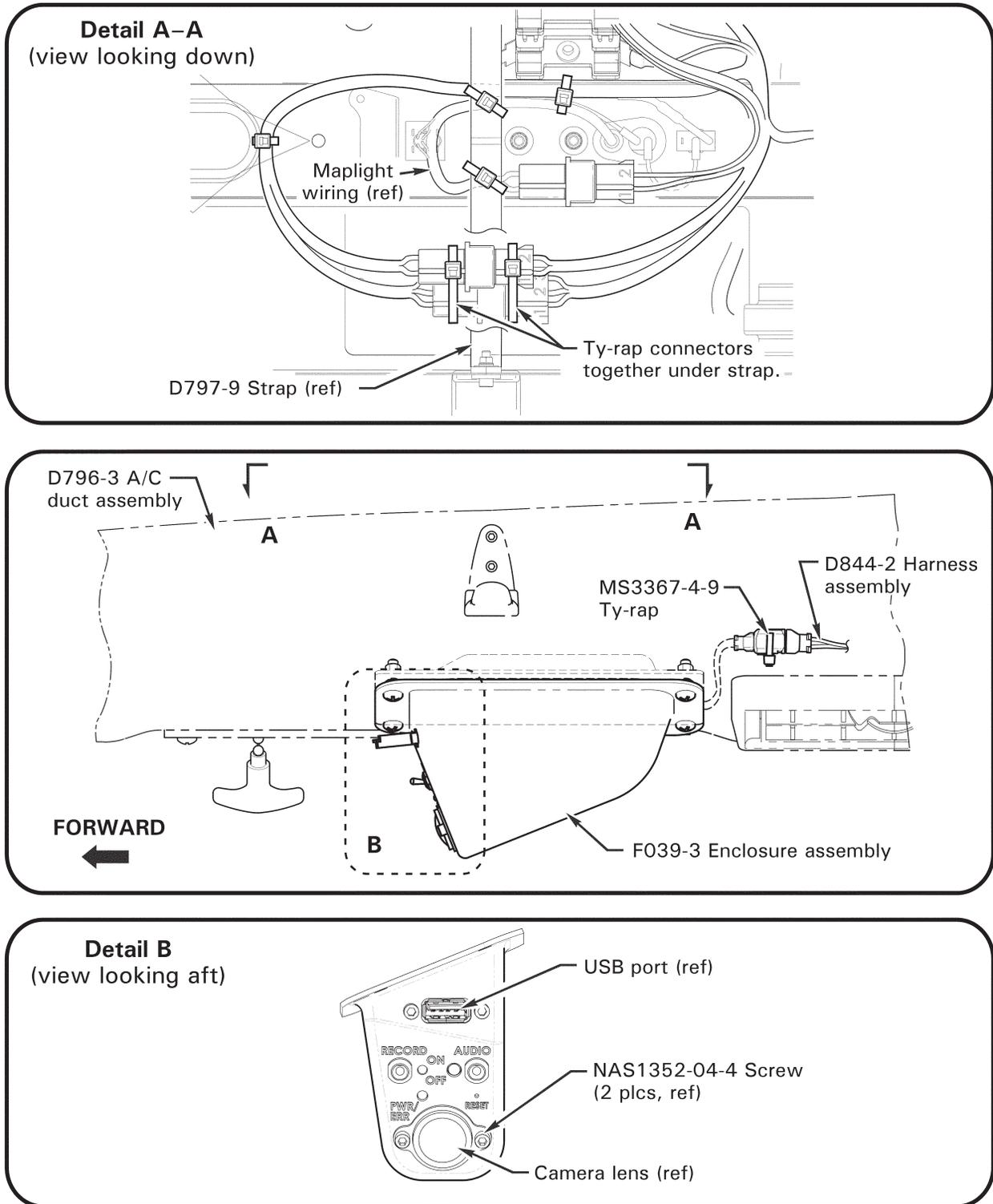
**FIGURE 2** Connecting camera to D844-2 harness
