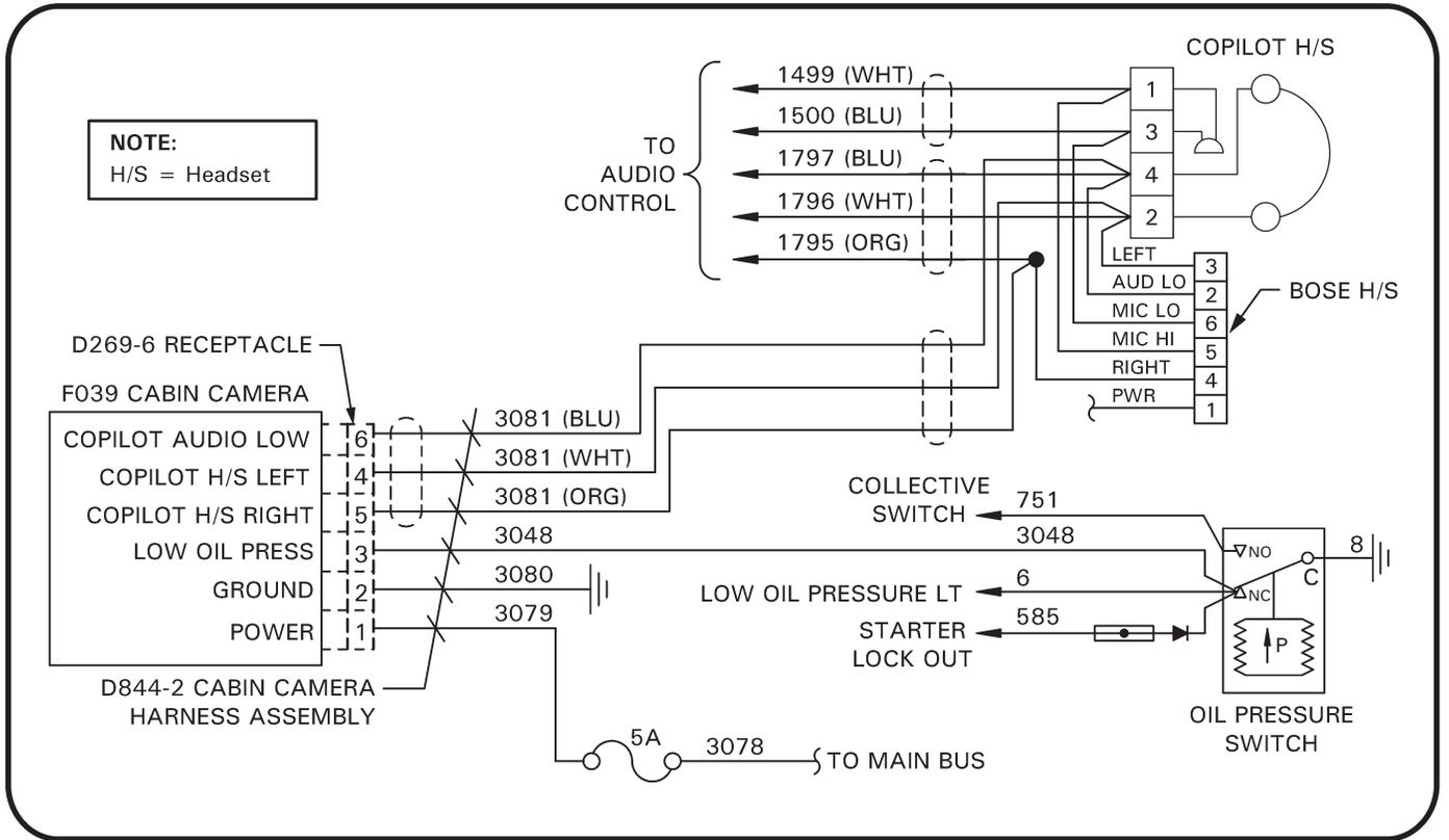
**FIGURE 1 Wiring schematic**
