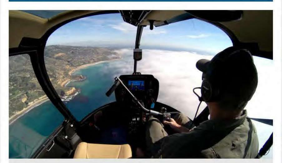
Robinson's Cockpit Video Camera introduced at Heli Expo 2020 is now optional on R22/R44 helicopters and standard on R66 helicopters ordered after 15 January 2021. Securely mounted in the ceiling for minimal vibration and optimal field of view, the 4K Ultra HD video camera records video, intercom audio, radio communications, and GPS position to a removable 128 GB USB flash drive.
