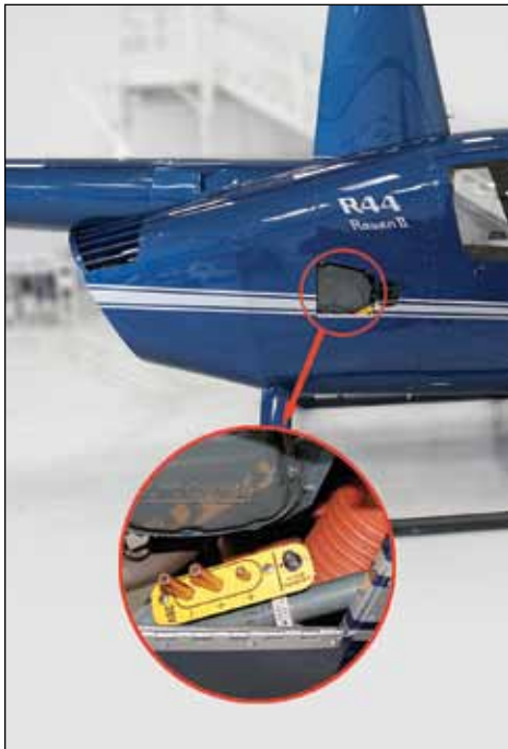
The optional MS3506 external power receptacle installed in a R44 Raven II.
