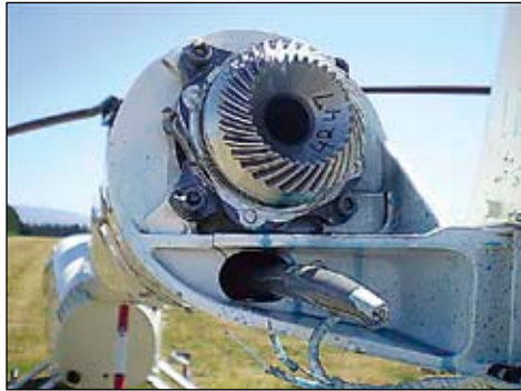
Little remained of the tail rotor and tail rotor gear box following the accident.
