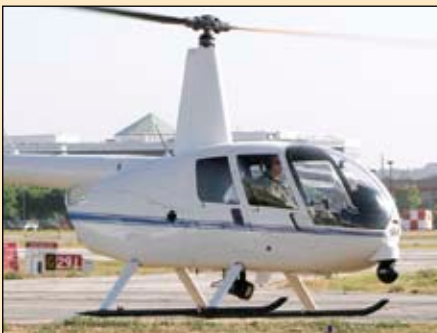
The Raven II Police Helicopters are each equipped with FLIR system, searchlight, and moving map.
