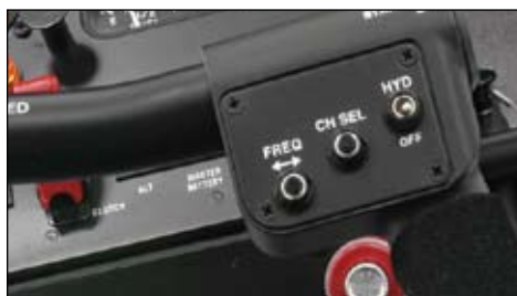
Cyclic grip controls allow pilots to switch COMM frequencies without looking at the console.
