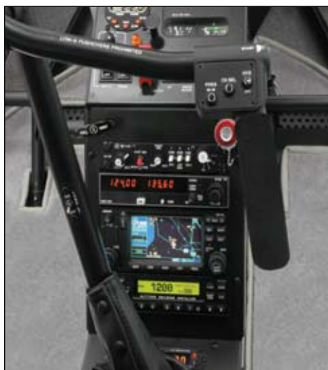
Center-mounted control panel and cyclic-integrated switches add to in-flight safety.
