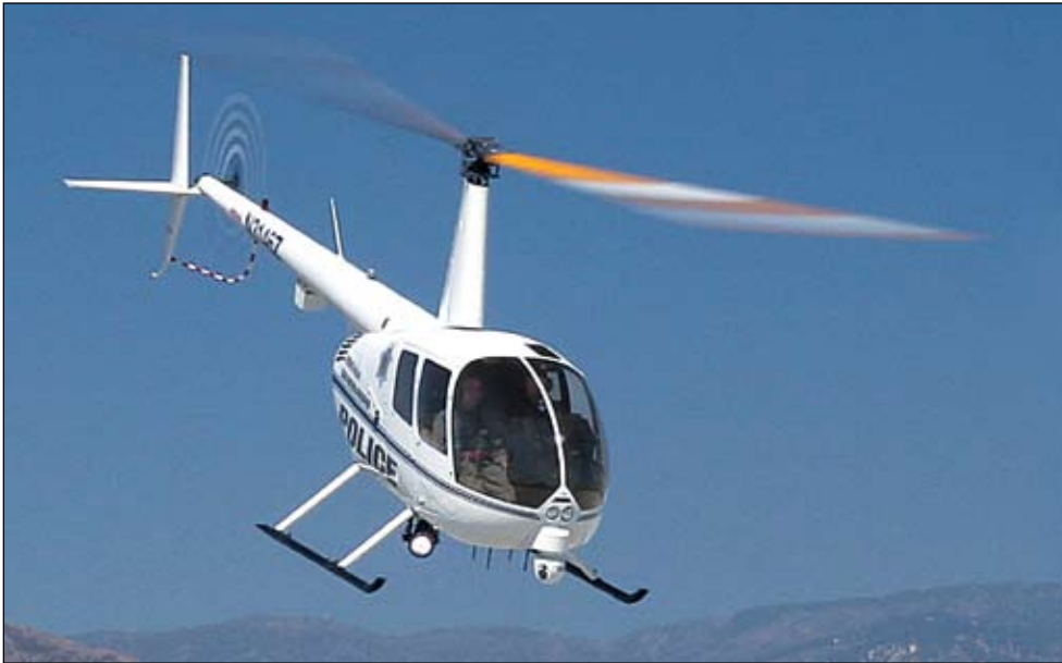
City of San Bernardino's R44 Raven II Police Helicopter equipped with FLIR sensor and spotlight.
