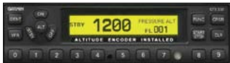
Mode S transponders broadcast more accurate flight data to improve air traffic communications.
