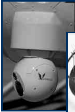
R44 Police Helicopters include Inframetrics 445G-MKII Infrared Sensor and Camera (above left) and Spectrolab SX-5E Searchlight (above right) as standard equipment.
